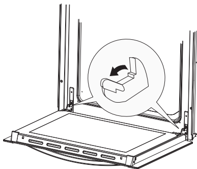
Tilting the hinge safety catches
